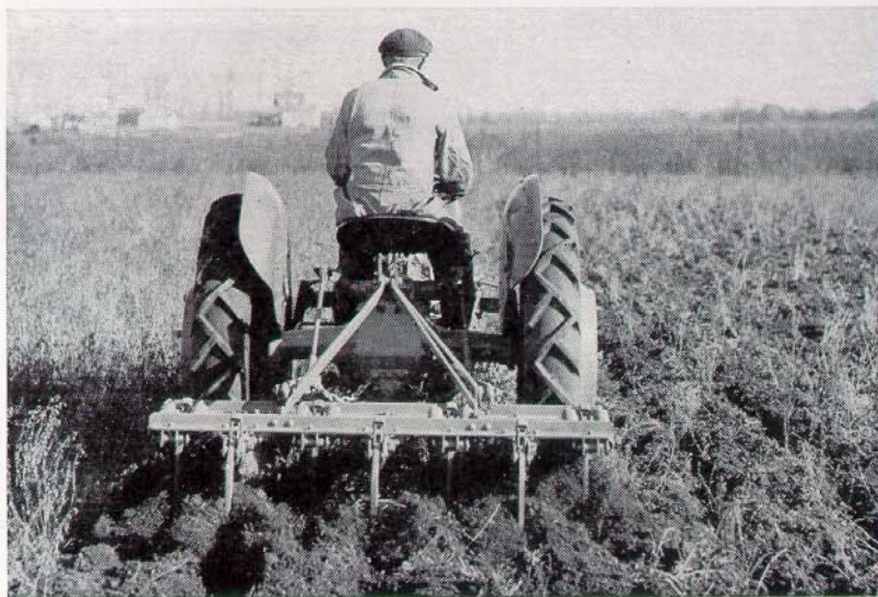
19 Aerating and preparing stubble land with a unique new implement — the Ferguson General Cultivator. This implement is equipped with a new type of spring tine which will cultivate the hardest land, but at the same time will ride over an obstruction, such as tree roots, without stopping the tractor or damaging the implement.
