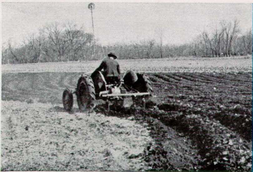
15 Contour middlebusting. The implement is outstandingly good for this kind of work because of its unique connection with the tractor. Suitable planter attachments are available.
