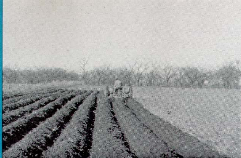
14 The Ferguson middlebuster is constructed of the highest grade alloy steels and is indestructible in the worst conditions. There are adjustments from 36 inches to 42 inches to cover all requirements.
