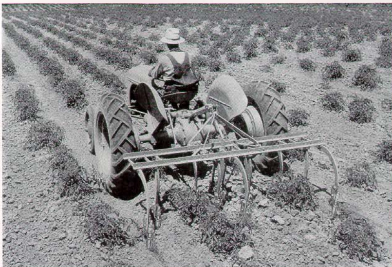
9 Cultivating tomatoes — one of the many cultivating jobs which can be done with the universally adaptable Ford Tractor with Ferguson System.
