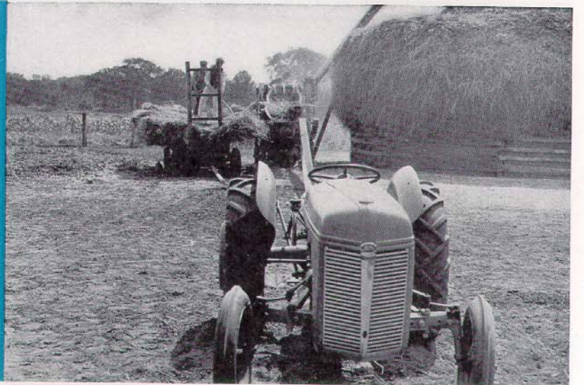
24 Ample belt power for all farm conditions. Illustration shows Ford Tractor driving 22 by 36-inch separator.
