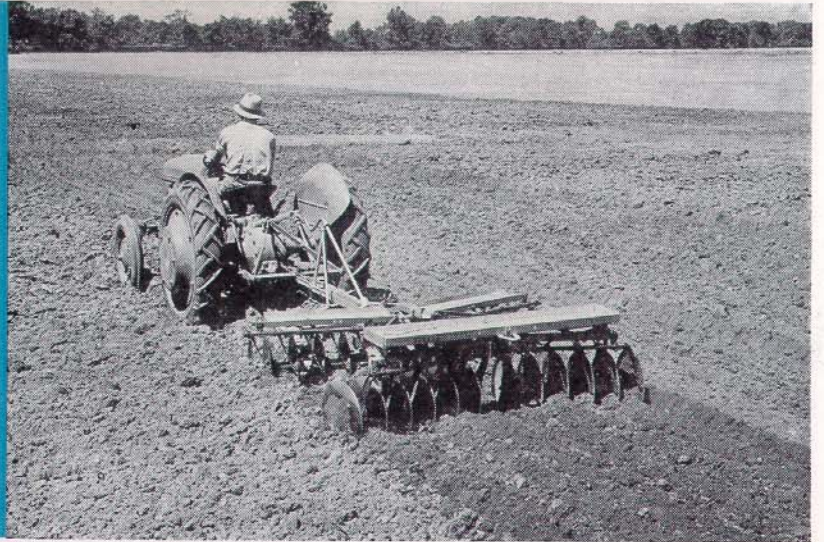
22 The tractor can be used for pulling the farmer's ordinary horse-drawn disc harrow. Or, as illustrated, it pulls easily the ordinary type of tractor disc harrow.
