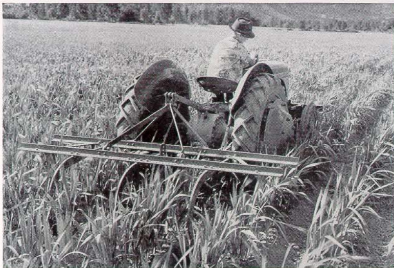
11 Young boy cultivating gladioli. Ferguson unit implements can be attached or detached with ease in about one minute and without the use of any tools.
